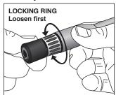
the *knob* to the desired position. To shorten, firmly hold the barrel and unthread the *locking ring* to the desired position. Finally, thread the locking ring or knob together and tighten. *NOTE: Extending the overall length may cause a loss of power.*
