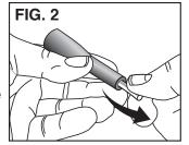
hose back (**FIG. 2**) into the knob until you see the tip of the brass fitting protrude through the side of the knob. This must be an air-tight fit, so you will have to pull somewhat hard (a few pounds, at least).
